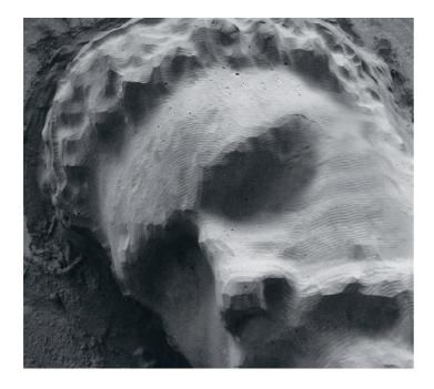
CNC-milling removes material layer by layer from roughing in the beginning to a fine and detailed resolution and its flexibility adapts to spatial structures and surface design.
