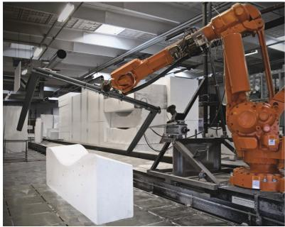
The process merges mass production manufacturing with customizable robot production technology. Hot-wire-cutting produces unique, single curved and ruled surface formwork by melting the EPS blocks in a pre-programmed hot-wire movement. Large-scale formwork is segmented, cut and re-clustered for post-processing and casting.
